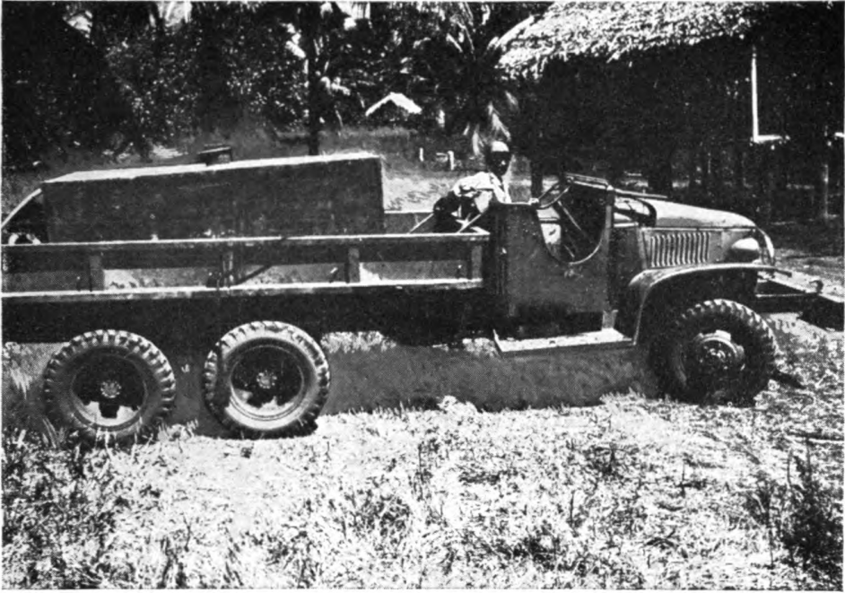
Figure 138. Steel tank mounted on 2½-ton truck for transportation of gasoline.
